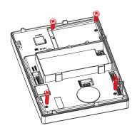
ii. Unscrew the PCB cover and remove from the rear of the front.
