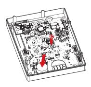
**iii.** Disconnect the piezo from the PCB and unscrew the PCB from the back.
