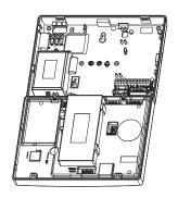
iii. Remove any cables connecting the back to the front half of the panel.
