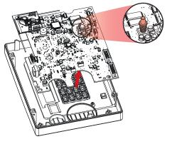
iv. Remove the PCB from the front of the panel. Note where the tamper spring is located to aid fitting the new one on the V11 PCB.
