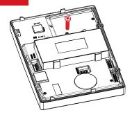
i. Unscrew the battery compartment and remove the battery.
