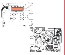
vi. Remove protective film from the LCD of the new PCB and the fit extra tamper spring supplied. Repeat steps 1-4 in reverse to put the new PCB in.
