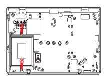
ii. Unscrew the PSU cover from the top and bottom and then remove the cover. Leave the PSU board in place.
