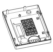
v. To prevent the keymat from falling out, is recommended to keep the front face down as this can be time consuming to put back in.
