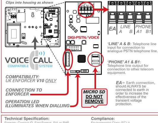
Formats: Contact ID. Fast Format, SIA or SMS Supports upload/downloading, Voice Calling functions Baud Rate: 1200bps Voltage: 12V.d.c. Quiescent: 20mA (In use: 40mA) Dimensions: 109 x 56 x 13mm Declaration of operation mode: Pass-through
